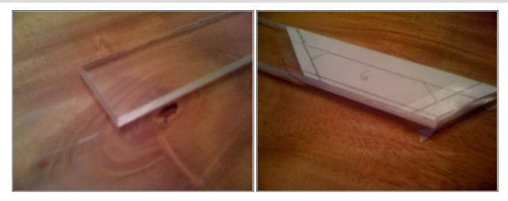
• Get some plexiglass and cut pieces to the shape of the LED segments. (I used the scroll saw for this.)
